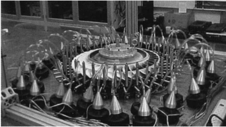
Fig. 2 CDFS mounted on the TEFF's traveling wave excitation system
